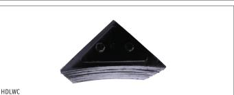
For maximum holding power, choose the **HEAVY-DUTY WHEEL CHOCK**. Made of reinforced rubber sheets that are laminated between thick steel end plates, it features a curved surface that really grips the road. A welded-on steel eye protects against loss. 11.5 lb. 11"L x 8"H x 6"W.
